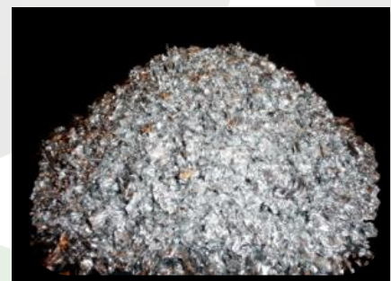
Recovered aluminium from the Enval Process
